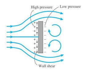
Drag force on a flat plate normal to the flow depends on the pressure only and is independent of the wall shear → Pressure Drag
