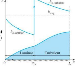
The average heat transfer coefficient (h) over the entire plate can be found by integrate the local Nu  $(Nu_x)$ :
