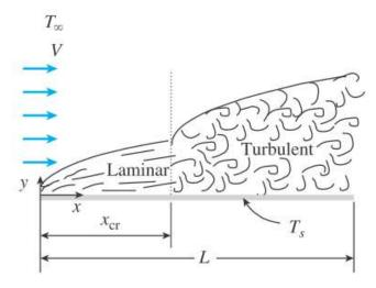
The Reynolds number at a distance *x* from the leading edge of a flat plate
