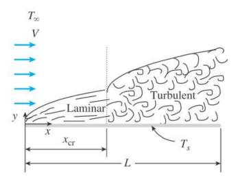
The average friction coefficients ( $C_f$ ) for the entire surface can be determined by integration from :
