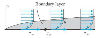
Drag force on a flat plate parallel to the flow depends on wall shear only → Friction Drag
