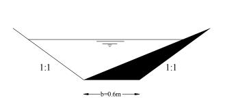
by using trial, we can get the critical depth  $(y_c) = 0.3m$ .
