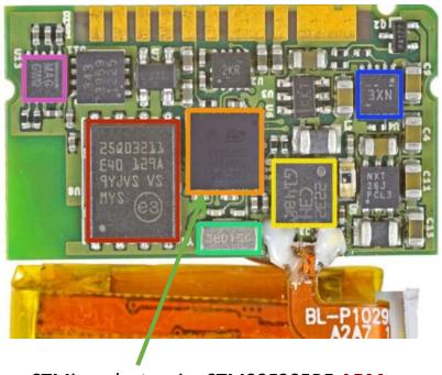
STMicroelectronics STM32F205RE ARM Cortex-M3 MCU, with a maximum speed of 120 MHz
