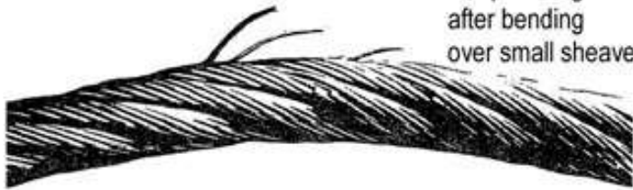
Rope break due to excessive strain
