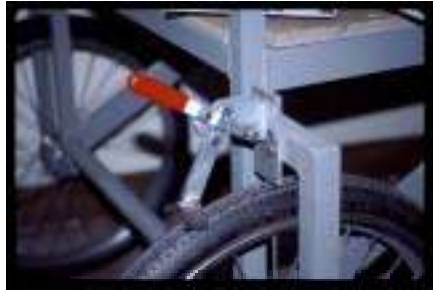
Brake for wheelchair. The mechanism exhibits a toggle motion
