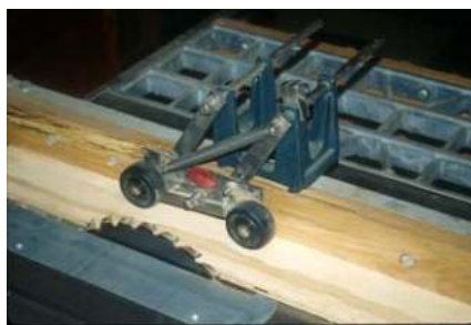
Kickback protector on table saw. The fourbar linkage is a parallelogram linkage.
