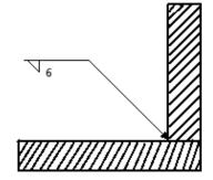
13. Calculate strength of the welded joint shown below, when 70 MPa is the allowable shear stress for the weld material.
