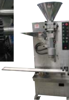
Automatic Packing Machine by New Max. KSS Spur Gears, segment shaped by secondary operation, are used at the crimping device.
