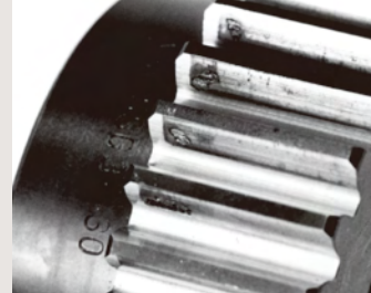
Poor tooth contact and pitting
