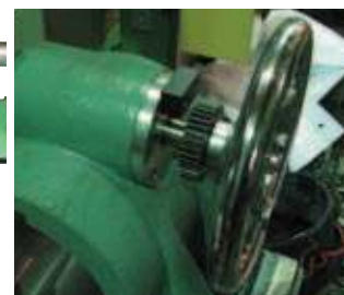
Electric Wire Winder by Sakuma Tekko KK. KSS Spur Gears are used at the stopper of handgrip.
