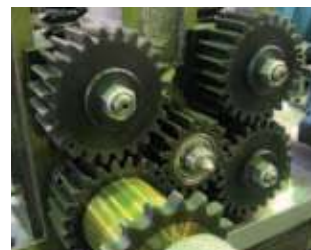
Takashima High-Speed Wire Straightening & Cutting Machines by Takashima Sangyo Co., Ltd. KSS Spur Gears are used at the feeder.
