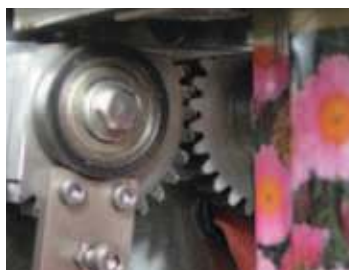
Automatic Packing Machine by New Max. KSS Spur Gears, segment shaped by secondary operation, are used at the crimping device.
