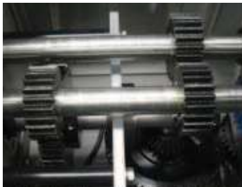
Full-automatic Forming Machine by Jey Machine Co. KSSA and KSS Spur Gears are used for stirring devices.
