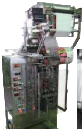
Automatic Packing Machine by New Max. KSS Spur Gears, segment shaped by secondary operation, are used at the crimping device.
