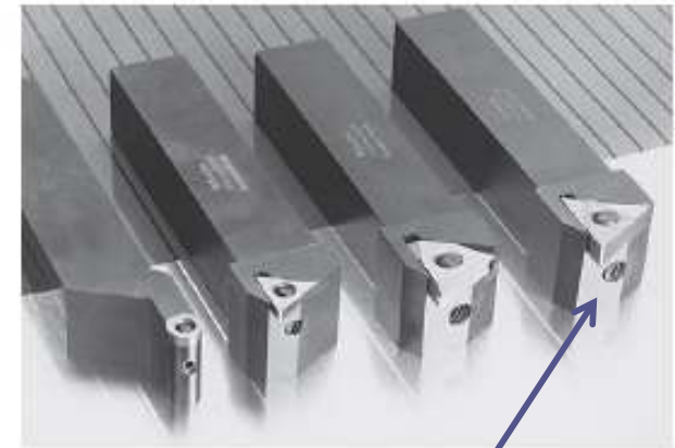
Inserts mounted with threadless lockpins (secured with side screws)
