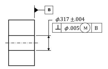
Calculate the geometric tolerance for cross sections in the system having the following sizes:
