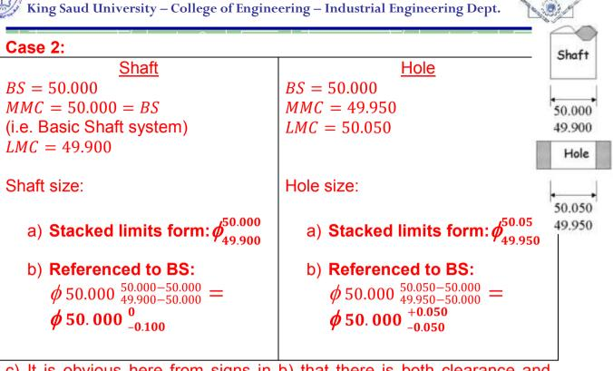
c) It is obvious here from signs in b) that there is both clearance and interference; thus,  $\phi_{49.900}^{50.000}$  $intereference_{Max} = MMC_{shaft} - MMC_{hole} = 50.000 - 49.950 = 0.050$
