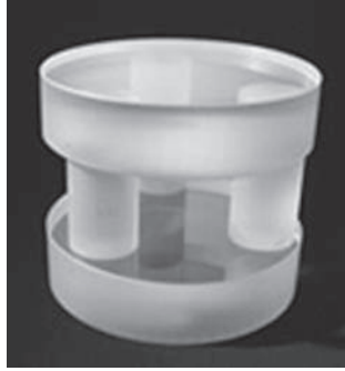
Left: Fused silica etalon. Right: A 10 GHz air spaced etalon with 3 zerodur spacers. (Courtesy of Light Machinery Inc.)
