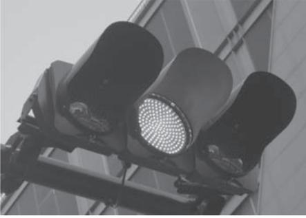
LEDs have now widely replaced the incandescent light bulbs in traffic lights.
