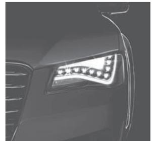
The Audi A8 uses LEDs for nearly all its lighting, including headlights. (Used with permission of Audi of America, Inc.)
