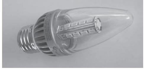
This LED-based light bulb for use in chandeliers uses a few watts of electric power (2.5W) to generate 135 lumens of light. There are 18 LED chips each with a yellow phosphor to generate the white light.
