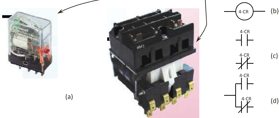
Fig. 5.13, a) Structure of electromechanical relay, b) Relay ladder notation, c) NO notation) NC notation and e) changeover contact notation.
