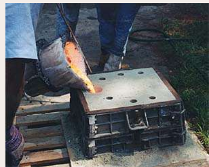
Open the mold and remove the pattern before pouring the metal
