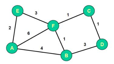
**Q1:** The routers in the network depicted by the figure above agree to use **distance-vector protocol** to build their routing tables. If **router A** just join the network with routing table only showing the cost to reach its immediate neighbors, how would the table of **router A** looks like after receiving the following tables in sequence: table of router B then table of router F then table of router E? (the received tables are shown bellow.)
