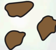
Rounded (atomization, chemical decomposition)
