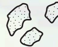
Porous (reduction of oxides)
