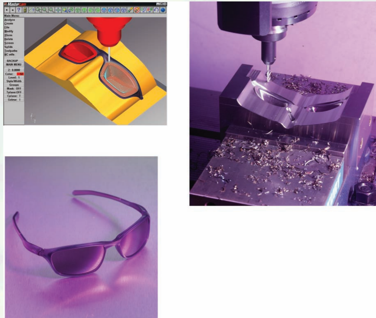
FIGURE 1.8 Machining a mold cavity for making sunglasses. (a) Computer model of the sunglasses as designed and viewed on the monitor. (b) Machining the die cavity using a computer numerical control milling machine. (c) Final product produced from the mold. Source: Courtesy Mastercam / CNC Software, Inc.
