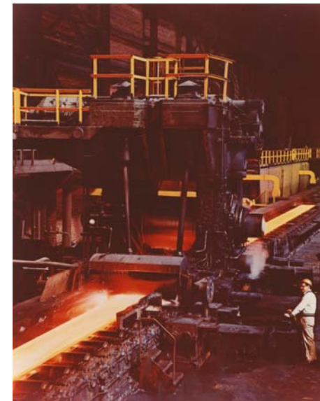
A rolling mill for hot flat rolling; (photo courtesy of Bethlehem Steel Company)
